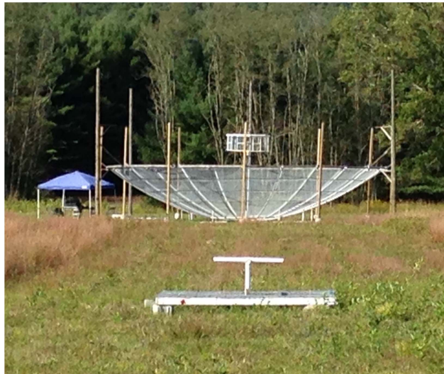
Figure 16. Left: the first of two prototype dishes at NRAO—Green Bank, used for measuring beam frequency structure with reflectometry and the beam pattern at 137 MHz by comparing satellite signals to the reference dipole in the foreground (Neben et al. 2016). Right: the measured EW power pattern plotted with dashed lines marking zenith angles of 20°, 40°, 60°, 80°.
