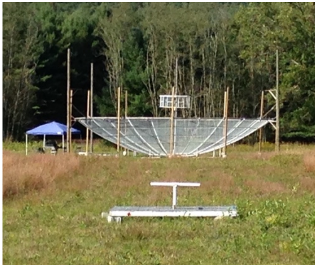
FIG. 4.— The dish with its suspended feed is seen in the back, 50 m north of one of the reference antennas used in the null experiment to study systematics. The experiment is conducted in Galford Meadow at NRAO–Green Bank.
