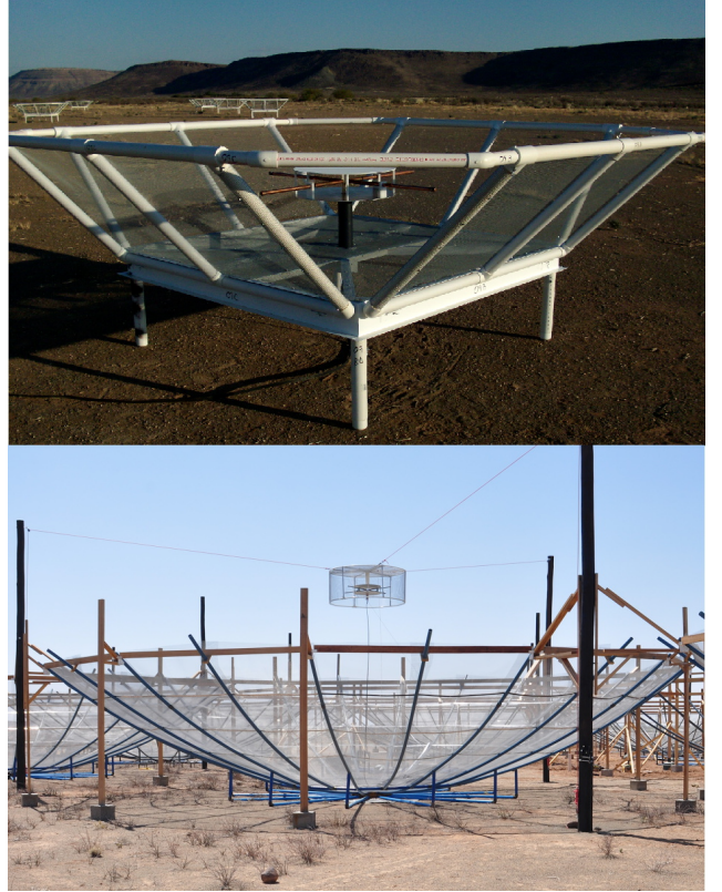
FIG. 1.— The HERA antenna element (bottom) uses a parabolic dish to achieve an order of magnitude increase in collecting area over the PAPER antenna (top). The sleeved dipole in the center of the PAPER backplane is identical to the sleeved dipole being suspended under the cylindrical skirt over the vertex of the HERA dish. The suspended feed arrangement has the potential to introduce intra-antenna reflections which we explore in this work.
