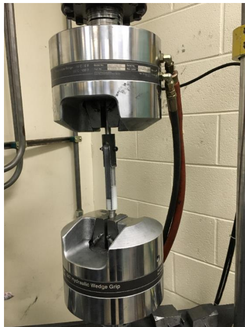
Figure 2: Steering Rack made with CBAM under Tensile Testing Equipment
