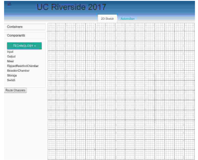
Fig. 4: Semi-automated design software initialized with available entities on the left hand side and an open drawing grid.
