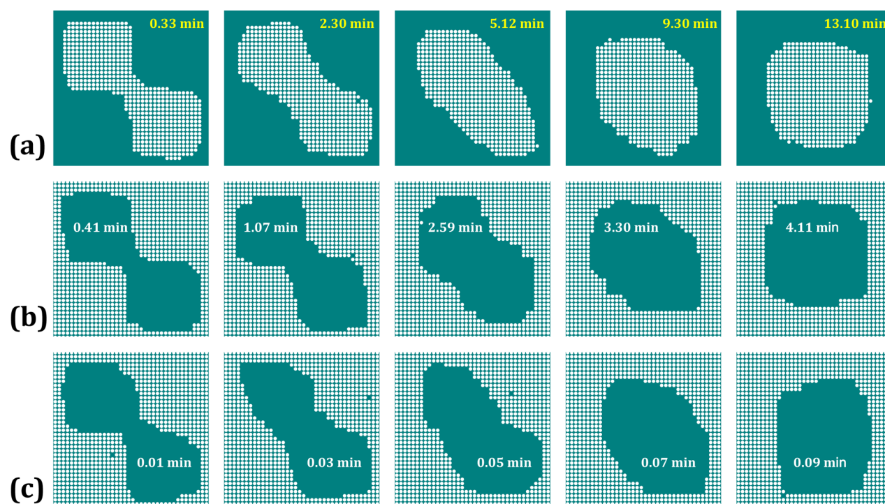
Figure 5. Comparison of KMC simulation results at 295 K for corner-to-corner sintering of (a) two 17 \times 17 atom islands, and (b) two 17 \times 17 vacancy pits. Cases (a) and (b) utilize our complete C4 + U4 model. Case (c) sets \phi_{t4} = \phi_{t5} = 0 .
