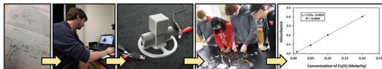
Figure 1. Undergraduate summer research interns drafted paper schematics for colorimeter instruments, which were translated into computer-aided design (CAD) files using accessible software packages. The digital models were fabricated into novice-friendly instrument kits for use in STEM laboratory learning activities at the introductory level.
