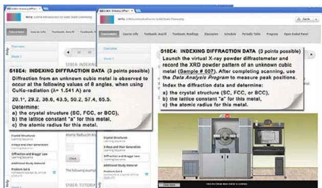
Figure 3. The screenshots of assessment pages of the undergraduate MITx course “Introduction to Solid State Chemistry” available on the MOOC edX platform. MIT Students had to determinate the crystal structure, lattice constant and atomic radius of an unknown cubic metal. Before the integration of v-XRLab (left) students were provided with the diffraction peak positions ready to be used for calculations. After the incorporating v-XRLab, students were provided with a sample number, randomly generated by the system. They had to become familiar with the equipment, perform all procedures required in the actual hands-on experiment, measure peak positions, and only after that, were they able to calculate the required parameters.
