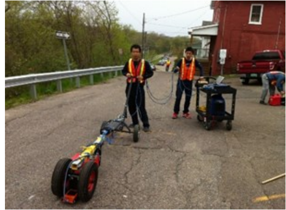
b. Dual-band GPR instrument on Railroad Ln.
