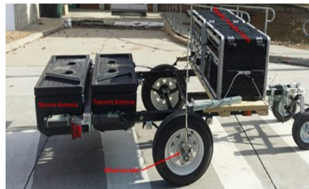
b. GPR cart with multi-static array
