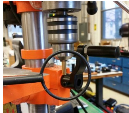
b. Magnet in drill press with electromagnetic probe
