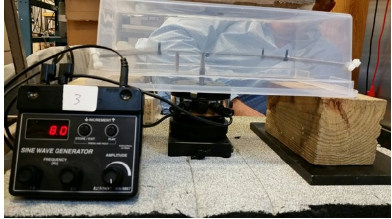
b. Plate with array vibrating at 80 Hz
