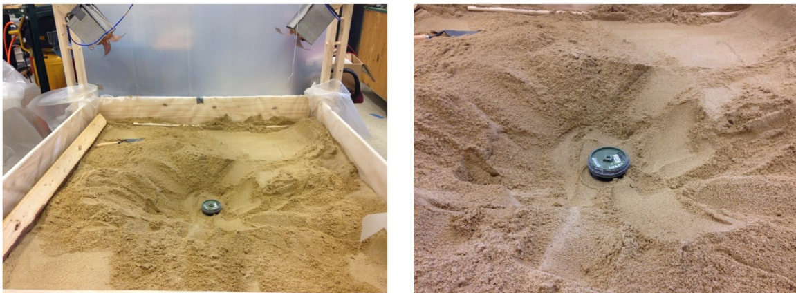
Figure 19 Buried object with non-uniform top surface in sandbox testbed
