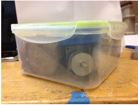
a. Rotating magnet transmitter in water tight box with rocks.
