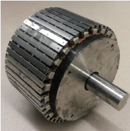
Figure 5: Fully assembled inner magnetic gear with outer control rotor shown [16]
