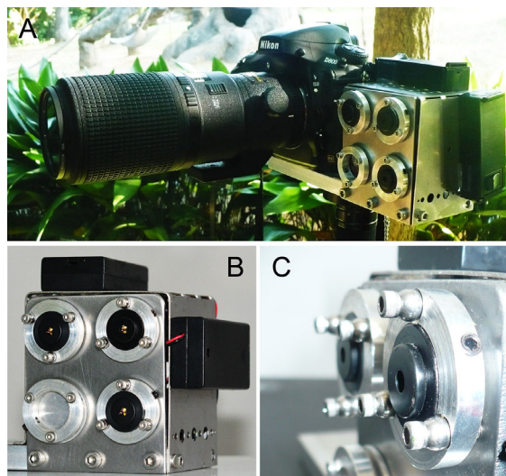
Fig. 2. Photogrammetric kit, including a digital SLR camera and housing for three parallel lasers mounted onto a steel base. Separate AA battery packs for each laser module are mounted on the outside of the laser housing (A). The parallel laser housing allows for positioning of four laser modules for flexibility. Only three modules are used here. (B). Close-up view of the aluminum collar surrounding each laser module (C).
