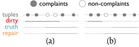
Figure 4: Graphical depiction of correct (a) and over-generalized (b) repairs. Solid and empty circles represent complaint and non-complaint tuples. Each thick line represents the interval of query q 's range predicate. Dirty: incorrect interval in corrupted query; truth: correct interval in true query; repair: interval returned by the solver.
