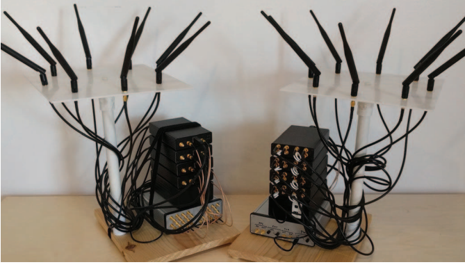
Fig. 3. 8-antenna experimental testbed based on Ettus USRP B210 software defined radios.
