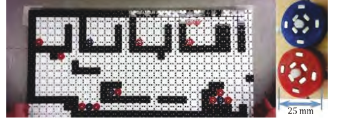
Fig. 9. A macro-scale demonstration of particle assembly using gravity as the external force and magnetic attraction between red and blue particles for assembly. Inset shows details of the magnetic sliders with magnets of opposite polarity facing outwards. See video attachment for a demonstration.
