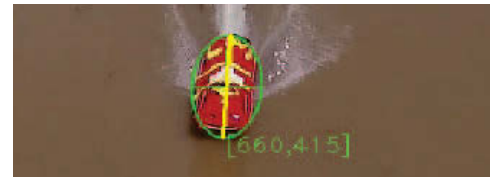
Fig. 9. EMILY localization using histogram back-projection and CamShift algorithm during the second trial. Green cross represents the centroid, the ellipse approximates the shape, and the yellow line represents the orientation.
