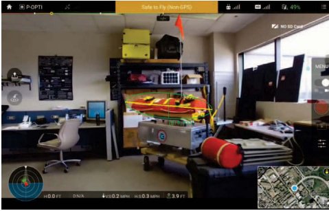
Fig. 12. Testing the reliability of position and orientation estimations under various viewpoints. View from UAV.
