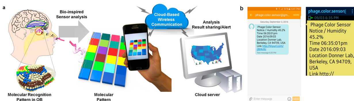
Figure 5. Schematics of smartphone-based sensor analysis system. (a) Schematic of perception of smell. When odorant molecules come to the surface of an olfactory membrane, they activate multiple cross-reactive receptors that transfer a unique combination of signals through neurons to the glomeruli of the olfactory bulb (OB). Colorimetric fingerprints from cross-reactive phage color sensor arrays can be analyzed in a similar manner. Images of phage sensors that have been exposed to target analytes can be taken by a smartphone and uploaded to a server for analysis against a database of reference color fingerprints. (b) Screen captured images from Samsung Galaxy smartphone and Samsung Gear smartwatch exhibit the analytic and communication capabilities of our system during a live demonstration (Supporting Movie SM1). Through smartphones and wearable devices ( i.e. , smartwatch or smartglasses), these results are shared via SMS text messages, e-mail, or on social media and include spatiotemporal information with the location and date/time that the image was captured. Previous results are stored in the server, generating a comprehensive event history. The image of Samsung Galaxy and the captured images from Samsung Galaxy and Samsung Gear are used with permission from Samsung Electronics Co., Ltd.
