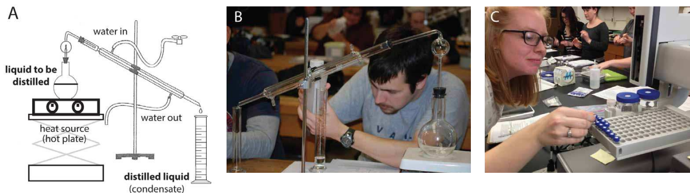
FIGURE 3. Distillation experiment and measurement: (A) Laboratory setup. (B) Student measuring initial water with distillation setup in standard classroom. (C) Student loading autosampler for Picarro water isotope analyzer.
