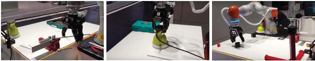
Fig. 5: Selected tasks implemented on the LBR iiwa using the CoSTAR system. From left to right: wire bending, polishing a surface, and collaborative structure assembly. For more videos see https://www.youtube.com/playlist?list=PLCv90iHF1jI3-VuVpUczGrNwvQOru3coZ
