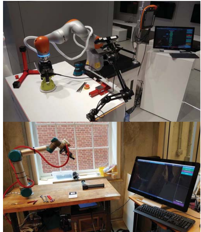
Fig. 1: The CoSTAR system set up to perform a wide variety of tasks. Top: CoSTAR running on a KUKA LBR iiwa at the Hannover Messe trade show. Bottom: CoSTAR running on a UR5 in a workshop.
