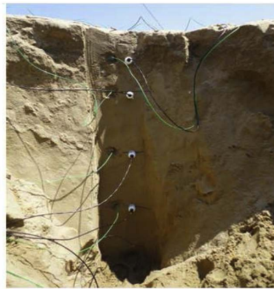
Fig. 2. Pictures of the: (a) plane view (with the sensor-based weather station tower); and (b) soil vertical profile (with three-needle heat pulse or TNHP sensors), of the study site.
