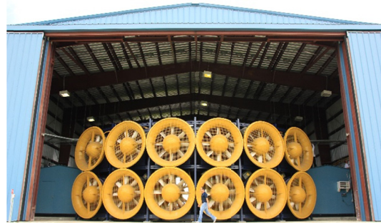
Figure 2. Full-scale experimental simulation of hurricanes with a 12-Fan Wall of Wind (WOW) facility (a NSF-supported Natural Hazards Engineering Research Infrastructure (NHERI) Experimental Facility (EF)).
