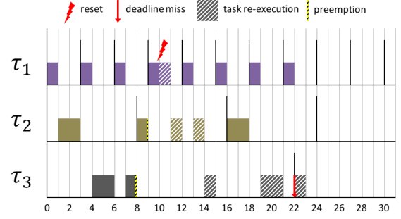
Fig. 1: Example of fully preemptive system with 3 tasks \tau_1 = (1, 3) ; \tau_2 = (2, 8) ; \tau_3 = (4, 22) , and restart at t = 10 - \epsilon ( C_r = 0 ). The taskset is schedulable without restarts, however, restart and task re-execution causes a deadline miss at t = 22 .
