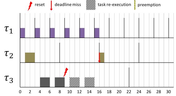
Fig. 6: Example of system with 3 tasks \tau_1 = (1, 3) ; \tau_2 = (2, 8) ; \tau_3 = (4, 22) , where \tau_2 and \tau_3 have a preemption threshold of \lambda_2 = 1 and \lambda_3 = 2 , respectively. Restart occurs at t = 9 - \epsilon ( C_r = 0 ). The task set is not schedulable.
