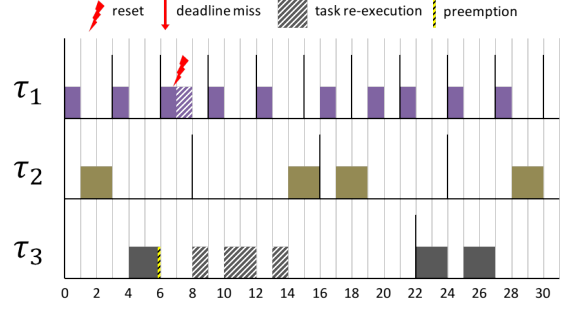
Fig. 5: Example of system with 3 tasks \tau_1 = (1, 3) ; \tau_2 = (2, 8) ; \tau_3 = (4, 22) , where \tau_2 and \tau_3 have a preemption threshold of \lambda_2 = 1 and \lambda_3 = 2 , respectively. Restart occurs at t = 7 - \epsilon ( C_r = 0 ). In this case, the task set remains schedulable.
