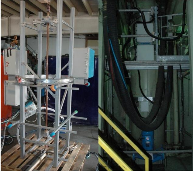
Figure 2 – Left: A single ring of the VARmetric™ measurement system undergoing calibration pre-installation. Right: VARmetric™ installed on a production furnace, with multiple rings to measure the arc as the ingot grows in the furnace.
