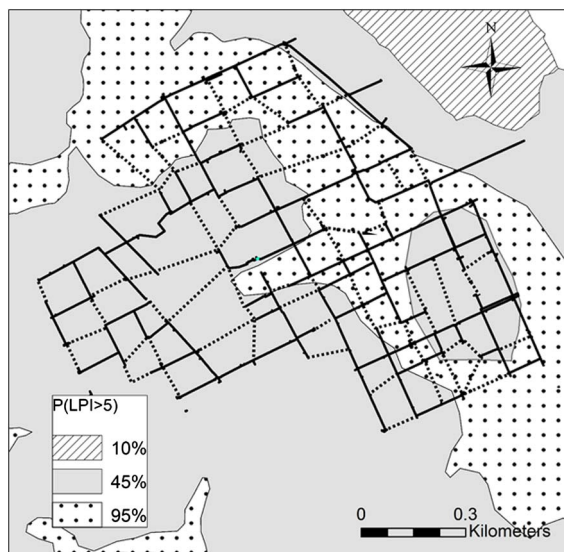
Fig. 6. CWSN layout overlaid on the liquefaction potential map of the region
