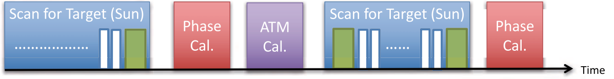
Figure 4. A cartoon of the observing sequences around a scan of a target. A box indicates the period of a scan. A scan is constructed from multiple subscans as shown in the “Scan for Target”. Except the scan for target, subscans are omitted in the figure. A red box indicates a scan for the phase calibrator; a blue box is the scan for the scientific target, and a purple box indicates a scan for atmospheric calibration near the target. White narrow boxes indicate subscans of observing the target, and green boxes indicate subscans of observing sky near the Sun with the attenuating levels for observing the Sun.
