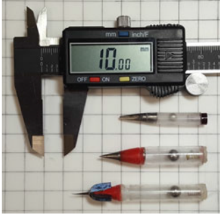
Fig. 2. Picture of three millirobot prototypes actuated by a magnetic hammer.
