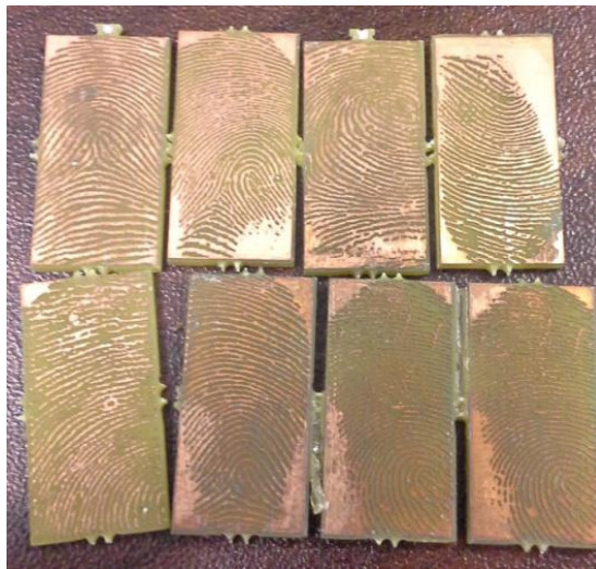
Figure 3: Etched fingerprints on PCB.
