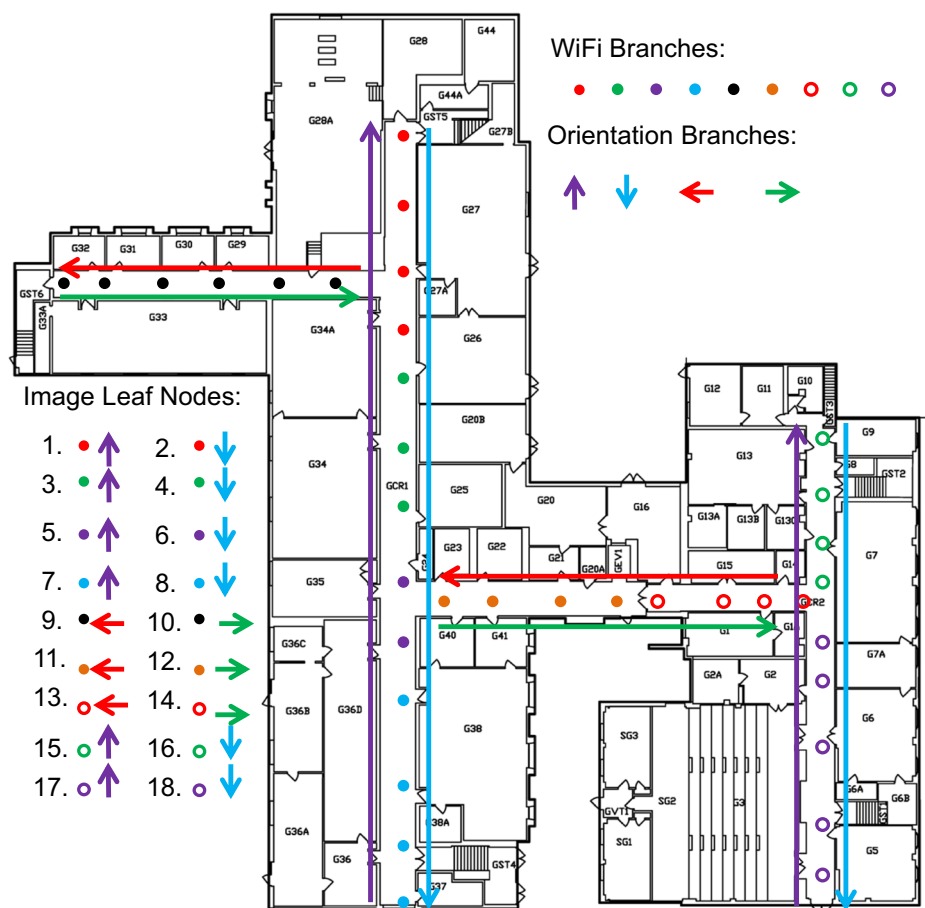
Fig. 11 Floor plan of a building with illustrations on how the signal tree is built. Circles are positions where we collect Wifi signals. Visual signals are collected from the beginning of each arrow to the end while sensor information is recorded simultaneously
