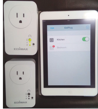
Fig. 1. Edimax plug and iPad installed with the control application
