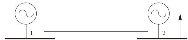
Fig. 1. Two-node, single-line transmission network for transmission-representation example.
