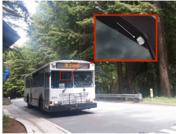
FIGURE 7 A UC Santa Cruz campus bus vehicle that was equipped with a Kontakt.io BLE beacon.
