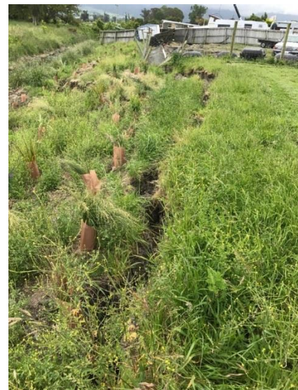
Figure 34: Lateral ground movements associated with vertical settlements in grassy area between Beach road and Lyell Creek. Note: Cracks are associated with vertical offsets and blocks have rotated away from the creek (-42.3902°, 173.6777°, taken facing N).
