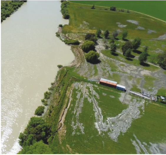
Figure 22: Aerial view of liquefaction manifestation at the Blenheim Rowing Club (Approx. coord: -41.4882^{\circ} , 174.0100^{\circ} , taken facing E). Photo: Marlborough District Council.
