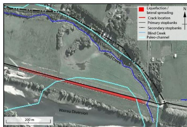
Figure 11: Overview of damage to the stopbank at Blind Creek. (Approx. coord. of centre of image: -41.442°, 173.978°)
