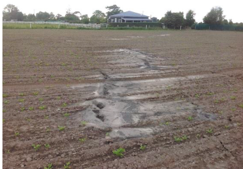
Figure 40: Liquefaction ejecta in the field south of Mill Road. The ejecta are concentrated in lines which continue in the background over a total length of ~100 m ( -42.3772^\circ , 173.6753^\circ , taken facing SE).
