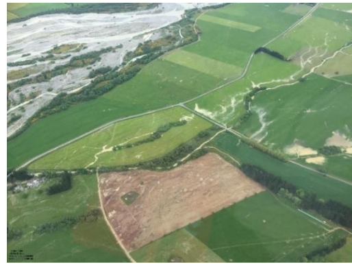
Figure 48: Standing water and ejecta west of Waiau town ( -42.638^\circ , 172.993^\circ ).
