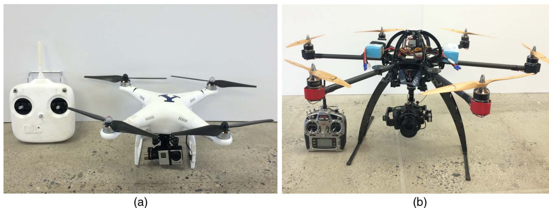
Fig. 4. sUAV platforms used in the post-liquefaction reconnaissance study including: (a) DJI Technologies Phantom II quadrotor with GOPRO Hero 3+ HD video recorder; (b) Aeronavics Limited Skyjib Super-6 hexrotor with Nikon D7100 DSLR camera with 35 mm AF-S Nikkor prime lens
