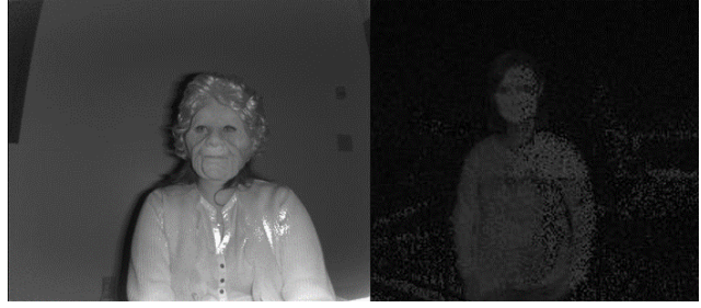
Figure 3: Illustrating low quality of the data captured in NIR spectrum in daylight. Image on the left is a good quality image captured indoors and image on the right is captured in daytime outdoor environment.
