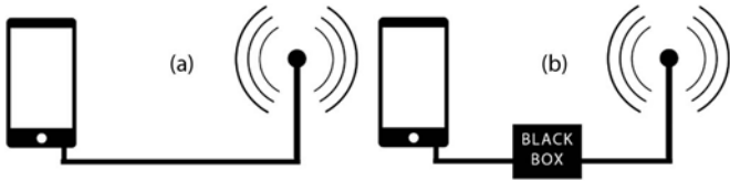
Fig. 5. (a) SP supporting V2V/V2I communication technology. (b) SP needing an external device (black box) for communication.
