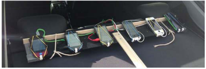
Fig. 2. Smartphones securely mounted in the trunk of a hatchback vehicle.
