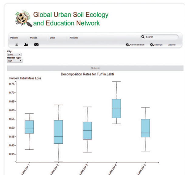
Figure 6. Example of data visualization on the GLUSEEN collaborative website. From the database Lahti, Finland was selected as city, and turf was selected as habitat. Boxplots show teabag mass loss after 6 months.
