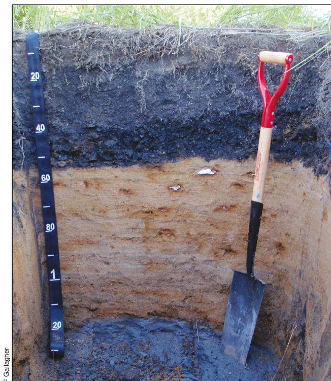
Figure 4. Soil profile at Liberty State Park. The A horizon is composed primarily of coal rock, and the soil horizon below is a compacted, low permeability fill layer.
