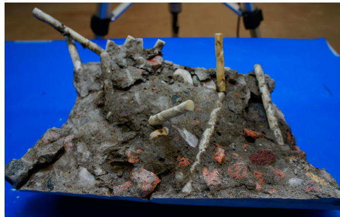
Figure 5. Distribution of the rebar (RB) needles in a cylindrical specimen tested for splitting tensile strength.
