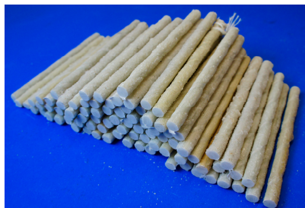
Figure 3. Needles obtained by cutting the scrap from producing GFRP rebars [28].
