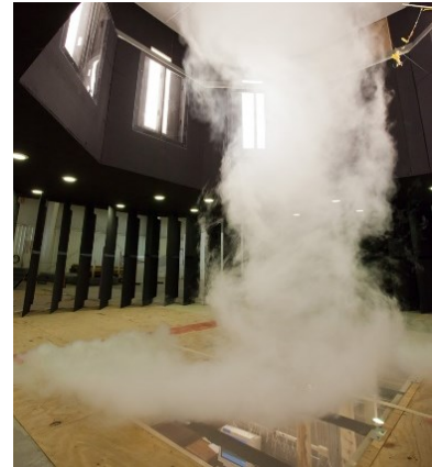
Fig 1 A Schematic illustration of the VorTECH simulator and a picture of a simulated tornado-like vortex.
