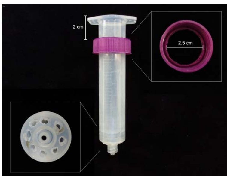
Figure 1. Tool for apoplastic wash collection. Apoplastic wash is collected by packaging whole Arabidopsis thaliana rosettes in a 30 ml syringe. Eight additional holes are melted into the end of the syringe with forceps to create channels for the wash to flow through. A 2.5 cm hole is punched out of a 50 ml conical tube cap. The cap is then slid onto the syringe 2 cm from the top. This allows the syringe to be screwed securely into a 50 ml conical tube. See Video 1.
