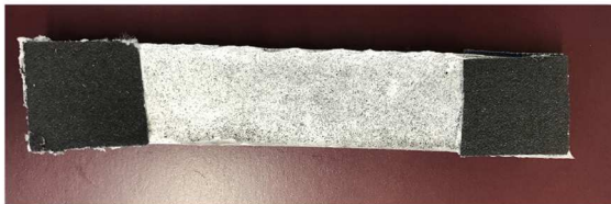
Fig. 12 (a) Dimensions of the rectangular sample and (b) the sample with sandpaper at both ends and random gray pattern on its surface
