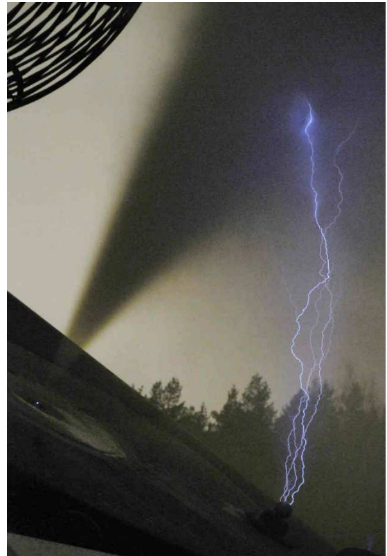
Fig. 7. Still picture (visible range; 5-s exposure) of negatively charged cloud (slanted jet-like, dark formation) and four upward positive discharges, about 1.5 m in length, triggered from the grounded sphere. Adapted from Kostinskiy et al. (3)
