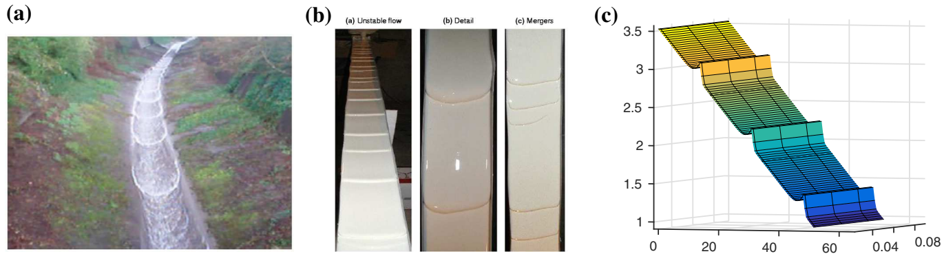
Fig. 1 Roll waves a on a spillway and b in the laboratory: pictures courtesy of Neil Balmforth, UBC. c Periodic profile of (1.1), F = \sqrt{6} , \nu = 0.1 , q = 1.5745 , X = 17.15 . For better comparison to experiment, we extended the profile here as constant in transverse direction
