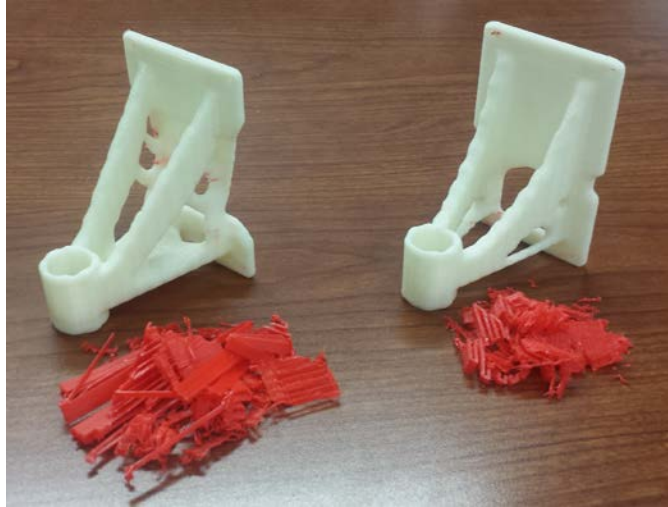
Figure 25: Printed mount bracket and the required support structures at 0.7 volume fraction.
