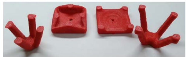
Figure 9: Tensile stool: tensile test, considering (left) anisotropic strengths and (right) stiffness.
