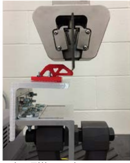
Figure 14: C-Bracket Fillet under compression. Test setup.
