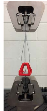
Figure 8: Tensile stool: tensile test setup for optimized stool designs.
