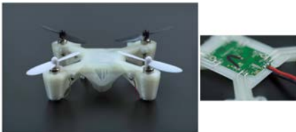
Figure 1: FDM printed functional quadcopter. Printed via Voxel8 with embedded electronics and endures structural loading [4].
