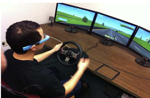
Fig. 2. Setup of the driving simulator with a participant wearing Google Glass.
