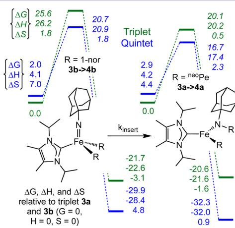
**Figure 5.** Triplet (green) and quintet (blue) surfaces for the  $\text{3b} \rightarrow \text{4b}$  and  $\text{3a} \rightarrow \text{4a}$  migratory insertions;  $\Delta G$  and  $\Delta H$  are in kcal/mol and  $\Delta S$  is in eu; transition states are in italics.
