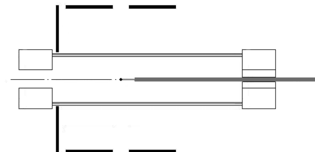
Figure 8: Schematic view of the testing setup. A sliding "needle" \alpha - source placed at the ANASEN axis.
