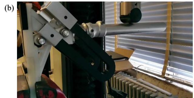
Figure 9: Experimental setup schematic (a) and photograph (b) measuring the ankle rotational stiffness k_{ank} , with F the applied load on the shank from the Instron with the foot constrained in a vice, M the resulting moment on the ankle and \theta_{ankle} the measured ankle angle.
