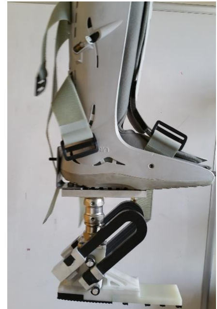
Figure 11: Pseudo-prosthesis boots mounted with the prosthetic foot prototype for preliminary testing
